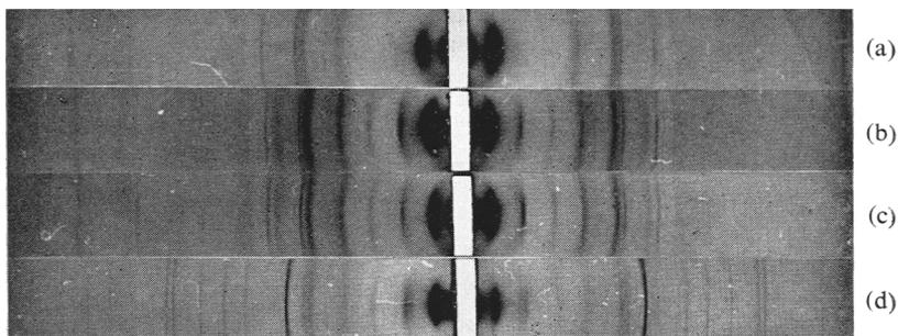
FIG. 1—X-ray patterns of flake aggregates treated with glycerol. Camera diameter 9.0 cm, radiation filtered Co  $K\alpha$ .
