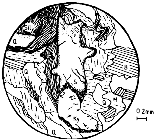
FIG. 3. Regional metamorphic gneiss (sample 177) showing grains of kyanite (Ky) and staurolite (S) within patches of fibrolitic sillimanite (Sill) and surrounded by muscovite (M), biotite (B), and quartz (Q). Inclusions of sillimanite needles can be seen within the upper part of the staurolite grain and within some quartz mosaics.
