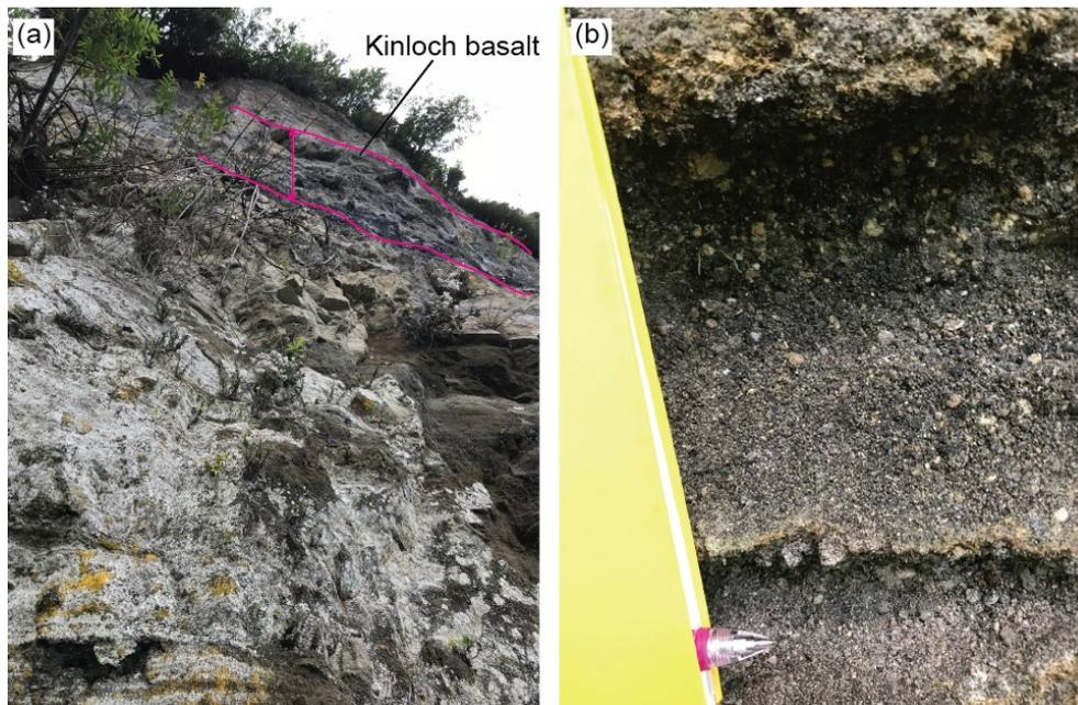
*Sampling of basalts in the TVZ: (a) Kinloch basalt that outcrops 20-30 m high in a cliff face, (b) sampling of basaltic scoria*
