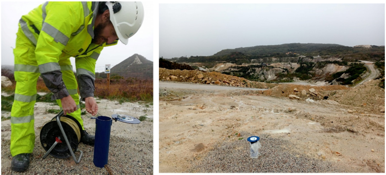
FIG. 3: FINAL DAY OF PLACEMENT MEASURING GROUNDWATER LEVELS IN THE TRELAVOUR DOWNS QUARRY USING A WATER LEVEL METER.
