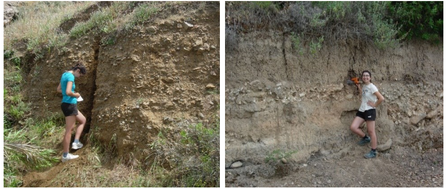
Figure 3 In situ luminescence profiling of an alluvial deposit (left) and an in situ gamma-ray spectrometer dose rate measurement of a fluvial sand deposit (right) for OSL dating.
