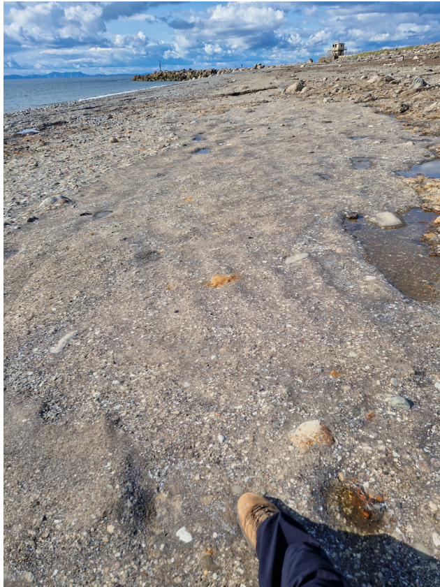
Figure 3: Bed top of a stratum of slag-dominated anthropogenic rock, Workington, UK. The whole foreshore in this photograph is cemented.
